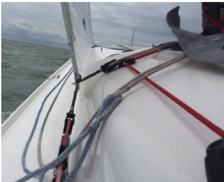
Jib clew shown In-hauled to about 1" from touching cabin house.
