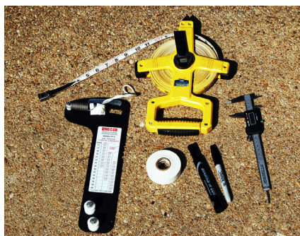
Tuning tools needed to accurately setup and tune your J/70 Another important setup tool is the use
