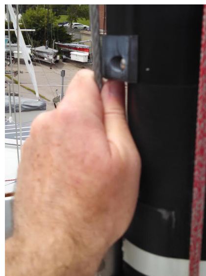
Hold main halyard to bottom of mast track to measure pre-bend
